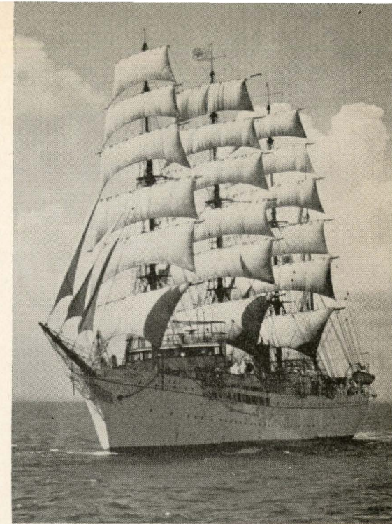
Japanese Training ship NIPPNO MARU under full sail. The ship is four-masted Bark with a gross tonnage of 2,285.77.
