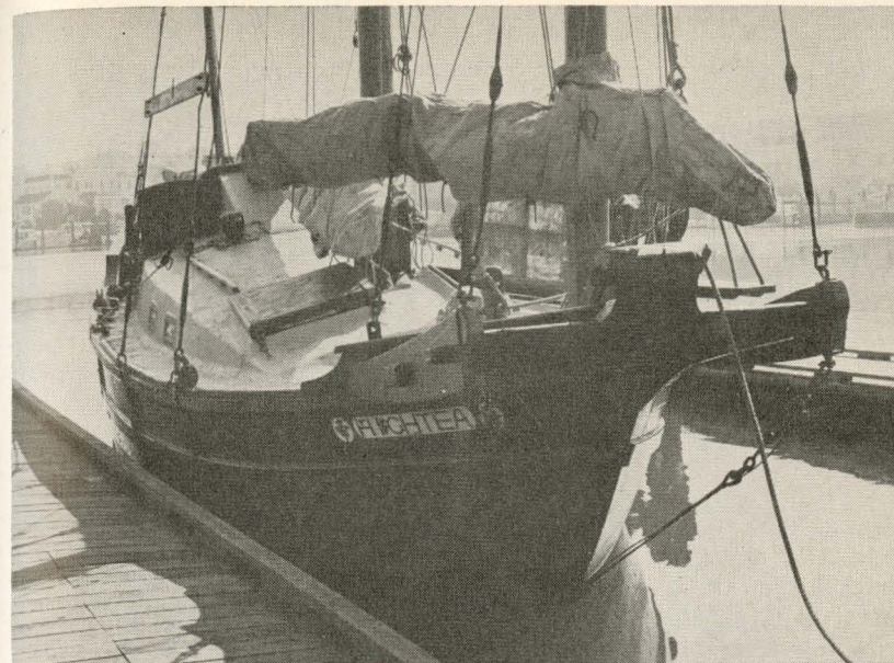
This view shows the sharp pitch of the High Tea's deck, which slants up toward the boat's typically Chinese high stern. Rigging on the bow acts to break some of the force of bow-on waves. Water quickly falls back into the sea from the tilted decks.
