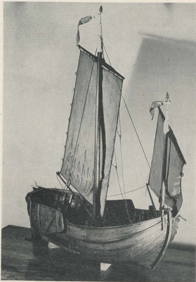
Looking like half an English walnut, the hull of this "Blänkenberghe Schuit" was so constructed that the adventurous North Sea fishermen of Belgium could run the vessel up on the beach when no port was available. This particular model, built in 1893, spent 60 years in the National Museum at Antwerp before being sent to the Marine Museum as the gift of King Badouin.
