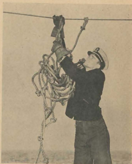
U. S. Merchant Marine cadet rigging scrambled rope above lifeboat for emergency use immediately after clearing port. Taken on a Liberty ship at sea.
