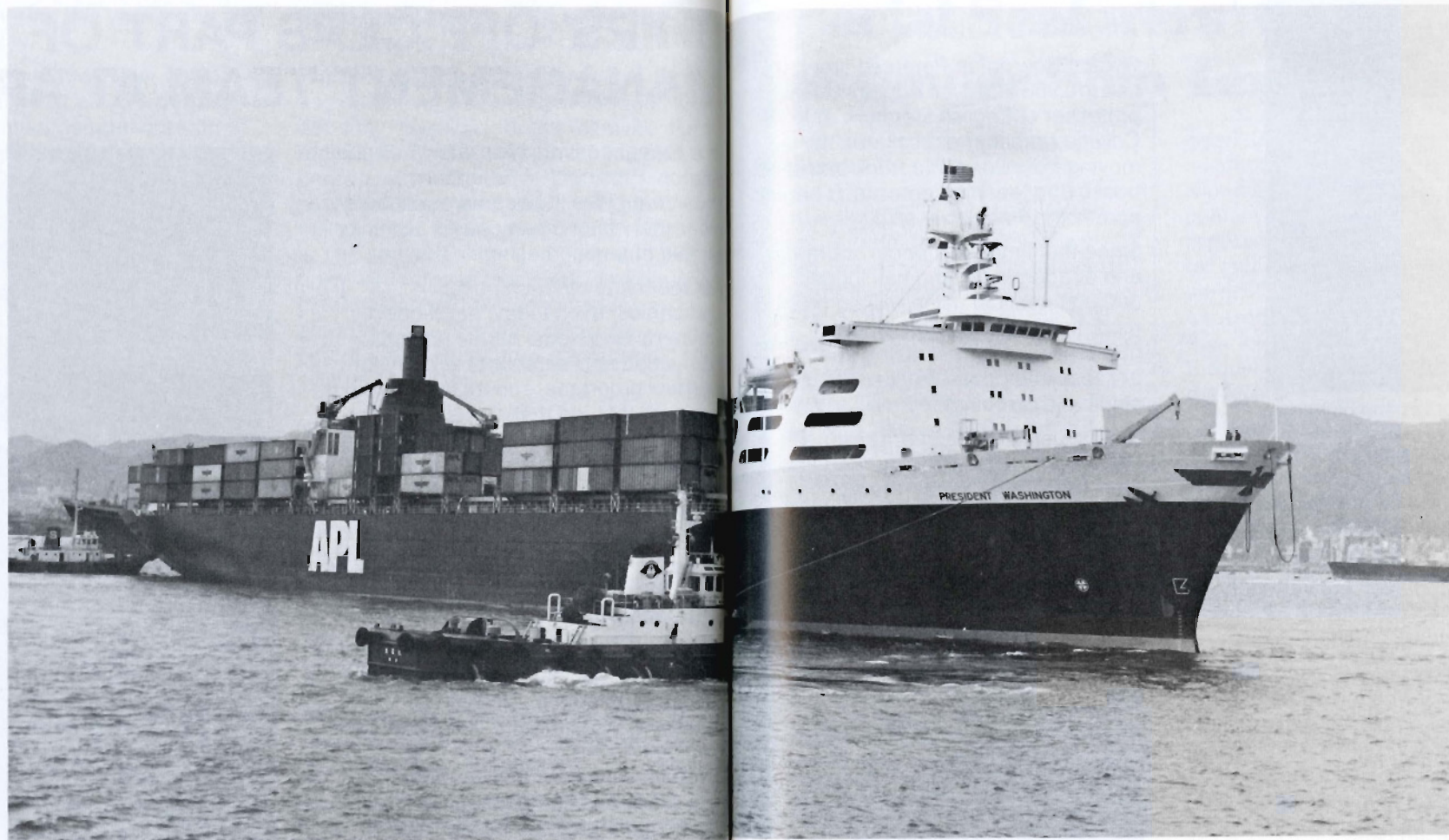
MV President Washington , one of APL's three C-9s, first U.S.-built diesel-powered containerships, and the largest. During the design phase, the company asked ship officers for their ideas on engine room, bridge, and other areas.
