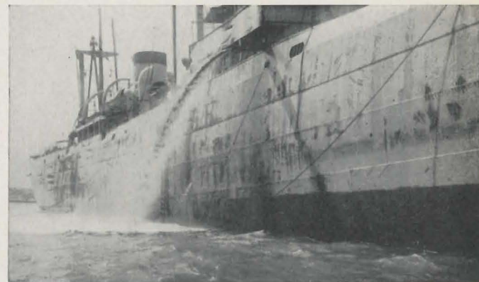
Pumping Water Out of No. 2 Hold
